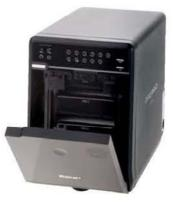
investigators to acquire multiple Suspect drives simultaneously, facilitate the transportation of evidence images from the field to the lab and to ensure the protection of valuable evidence data.
