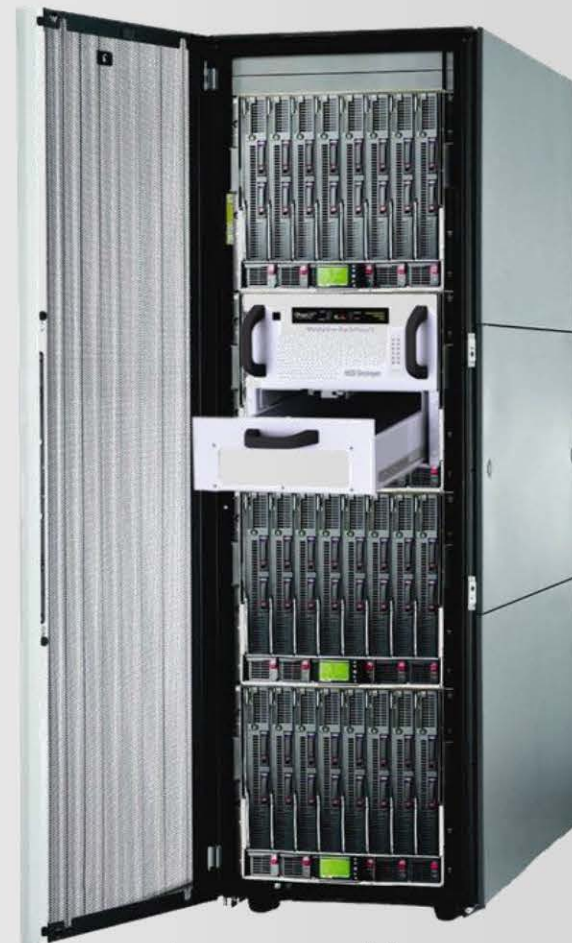
Phiston MVR-HDD installed in a standard 42U server rack
