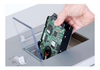
**STEP THREE** Remove the hard drive from the degausser unit and place it in the HDP feed chute. Hit the start button and a hardened steel punching die is driven completely through the drive.
