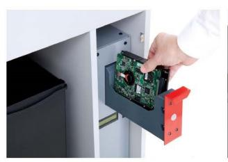
**STEP ONE** Drop a used hard drive into the slide-out drawer on the degausser unit. Most drives up to 1 ½" including full height, standard, and laptop drives are acceptable.
