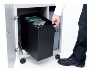
STEP FOUR Use the stider lever to drop the destroyed drive into the sturdy collection bin to await proper disposal. A weight sensor will automatically shut down the machine when the bin is full.
